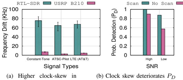
**Figure 3: Unpredictable clock skew makes frequency offset calculation harder resulting in poorer signal detection performance.**
