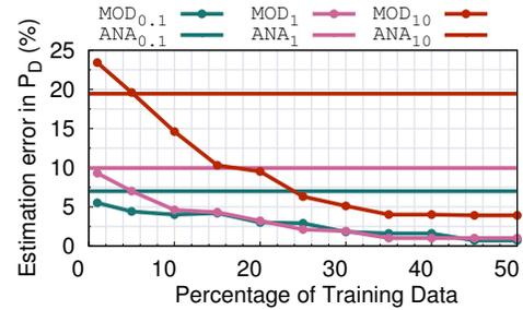
**Figure 7: Performance of the data-driven models  $MOD_{P_{FA}}$  compared to the analytical models  $ANA_{P_{FA}}$  for different values of  $P_{FA}$ .**
