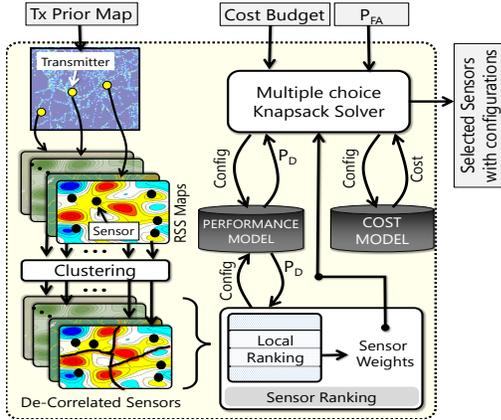
**Figure 10: Schematic of the sensor selection technique**
