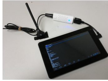
Figure 1: The DTV dongle with external antenna interfaced with the Android tablet.
