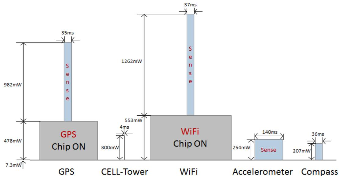
Fig. 8. Energy usage profiles for GPS, 3G, WiFi, accelerometer and compass.
