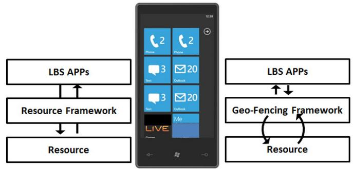
Fig. 2. Resource frameworks on smartphone. Current state of the art is on the left. The proposed solution is proactive and is on the right.
